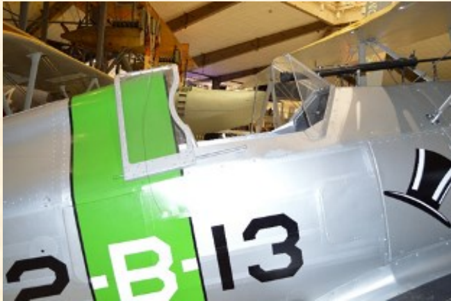
Right side of the cockpit and sliding canopy. The radio antenna wire can be seen running up from below the canopy.
