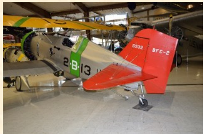
The layout of the tail section with the stitching of the fabric on the rudder particularly evident with the reflection of the light.
