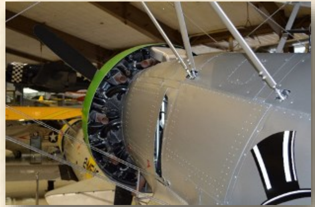
Details of the forward fuselage. The exhaust stacks coming directly off the engine cylinders can be clearly seen in this view.
