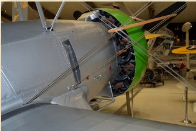
The right side of the forward fuselage. The wooden spreader bar on the flying wires can be clearly seen along with the short exhaust stacks on the engine.
