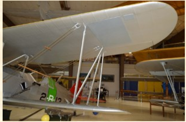
The left upper wing showing the strut arrangement and maintenance access panels on the lower surface of the upper wing. Also note the blue fairing on the bottom of the lower wing covering the aileron actuator mechanism.
