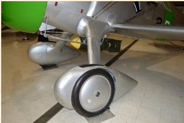
The left main landing gear. The black area on top of the wheel fairing appears to be a rubber step
