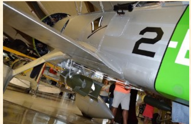
The fuselage bomb rack incorporates a trapeze mechanism for swinging the bomb clear of the propeller arc when dive bombing. Note the bungee cords running along the underside of the fuselage.
