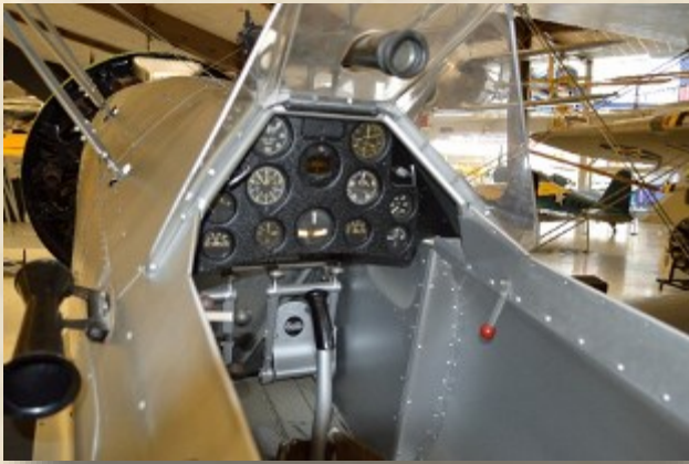
Cockpit interior. The optical sight can be seen protruding through the windscreen.
