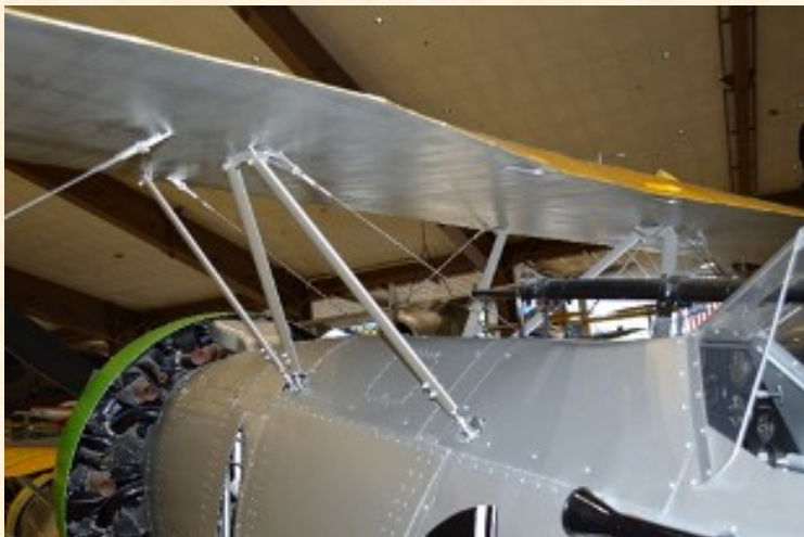
The cabane struts and bombsight. Note the protective cover on the front of the sight with a cable running along the top to open it in flight.
