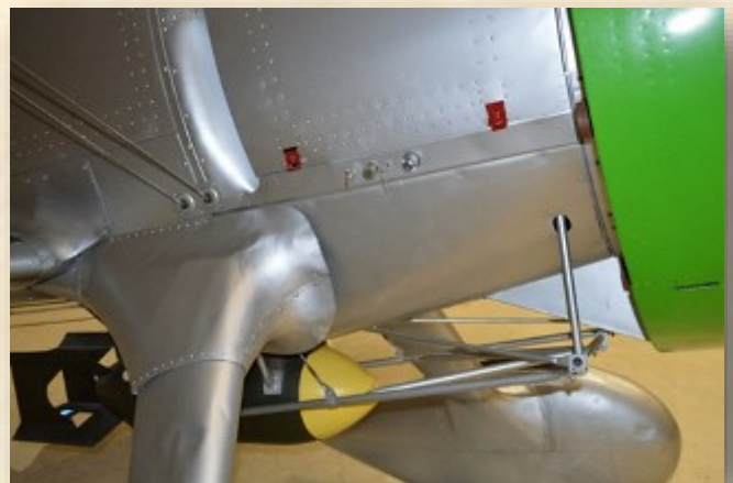
Right side of the forward fuselage and bomb trapeze. The attachment point for the inertial starter crank can be clearly seen between and slightly below the red cowl latches.
