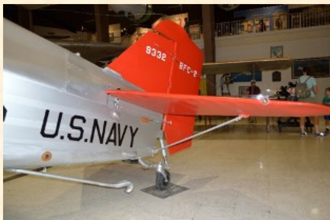
Left side of the tail. Note the light on the leading edge of the horizontal stabilizer as well as the radio antenna attach point on the top of the rudder.
