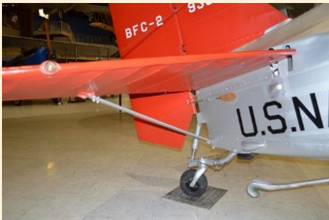
The right horizontal stabilizer and tail-wheel. Note the light on the leading edge of the horizontal just as on the left side.
